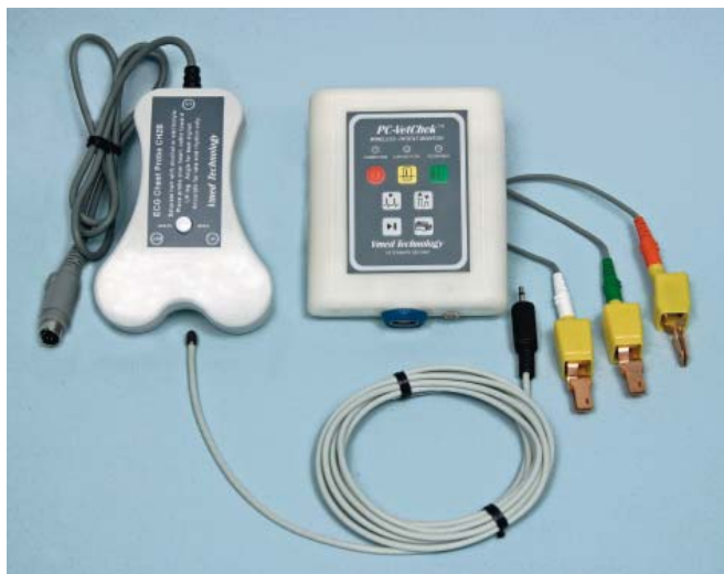
Low force ECG skin clips, ECG chest probe and temperature probe are included.
